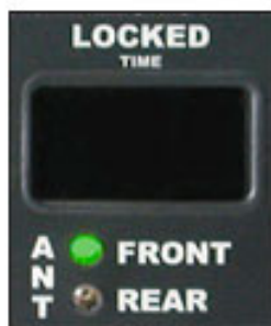
Figure 3.2.2.4b Antenna lights showing front antenna is active
