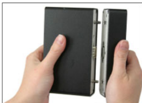
Figure 2.1a Separating the computer/display unit.
